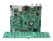
NVP1914C includes 4-Ch 960H video decoder and 5-Ch audio codec, which guarantees high quality images. It accepts separate 4 CVBS inputs from camera, TV, DVD and the other video signal sources. It digitizes and decodes NTSC/ PAL/COMET video signal into digital video signal which represents 8-bit ITU-R BT.656/1302 4:2:2 format with 27/36/54/72/108/144MHz multiplexed. Each video output can be selected between 720H and 960H. 5-Ch audio codec is 4-Ch PCM
